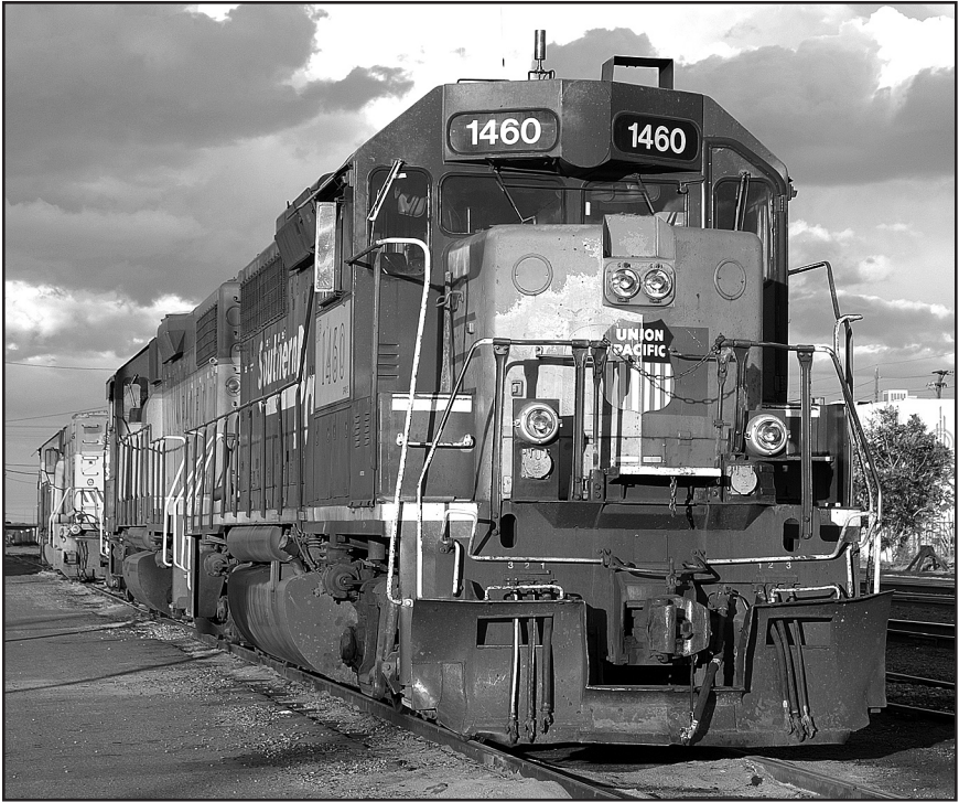
UP 1460 is an EMD GP40-2, built in March 1966 as SSW 7605. It became SSW 7965, and then got its Union Pacific number patch in December 2005. It was in the 36th Street yard in Denver on October 17, 2007. – Photo © 2007 Dave Schaaf.
